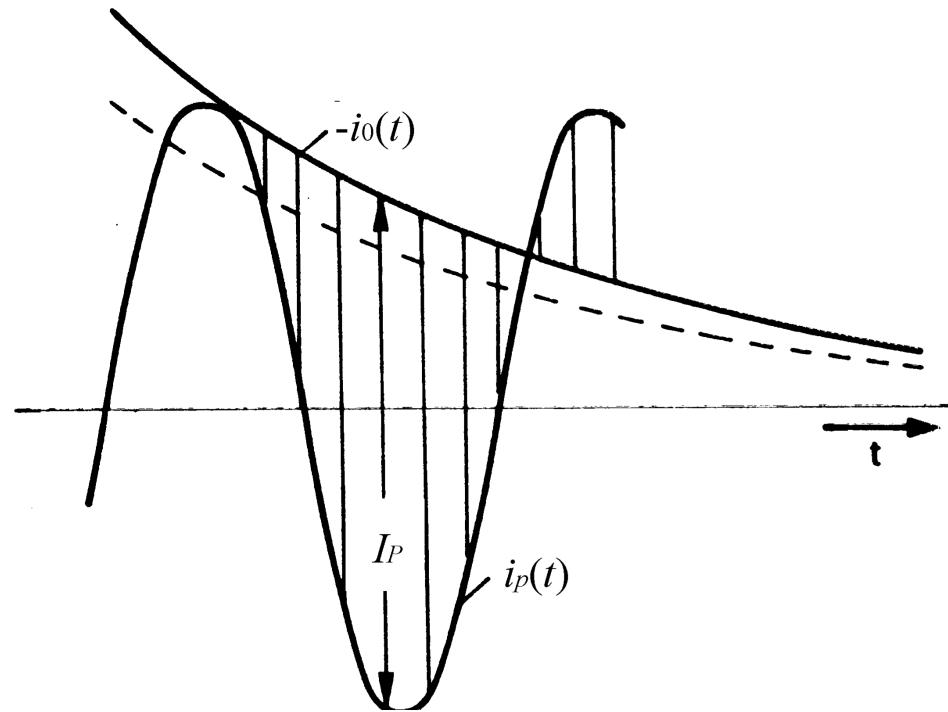
This equation is verified for  $\gamma=0$  and also  $\gamma=\pi \rightarrow$  **the largest value of  $I_p$**  is reached if the short-circuit occurs **when the voltage crosses zero, for any value of  $\varphi_{cc}$** .
